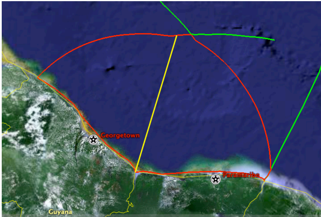
Figure 5. The division of the region in Figure 3 by the 17-degree line. The red curve outlines the entire region. The yellow line is a loxodrome with a bearing of 17 degrees. The green curves are extensions of the 200 nmi boundary and the Suriname – French Guyana equidistance line.
